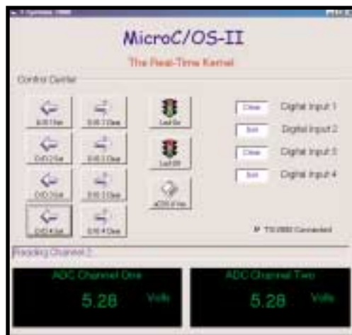
Photo 5 —This simple Visual Basic form provides an easy-to-use interface to the TS-2800 for software development.
