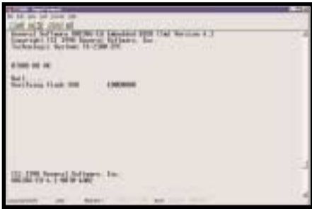
Photo 2 —The TS-2800 redirects all console activity to the COM2 serial port. Connect an ANSI terminal to COM2 and all text information that is normally displayed on a video screen is now displayed on the terminal window.
